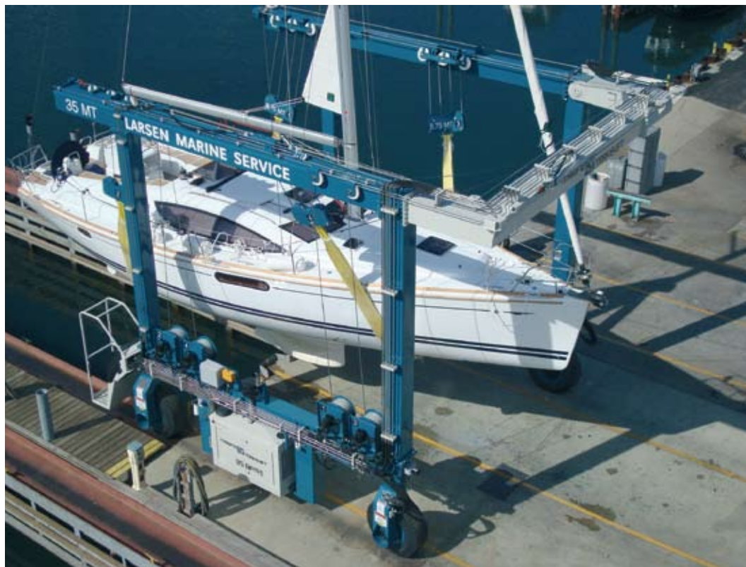
35 Tonne "Marina Travelift with extension beam to accommodate forestays on yachts, as ordered for Waikawa.
